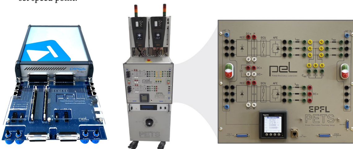
Fig. 1 PETS HIL (left) and actual PETS (right) that will be used for RT-HIL simulations and experimental investigations.
